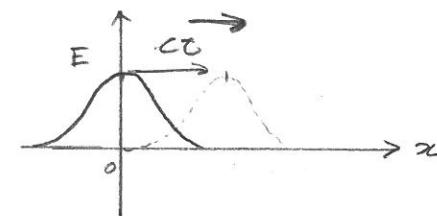
$$\omega = \frac{2\pi}{T} = 2\pi f = 2\pi \frac{c}{\lambda} = (k)c \quad \text{式}.$$
